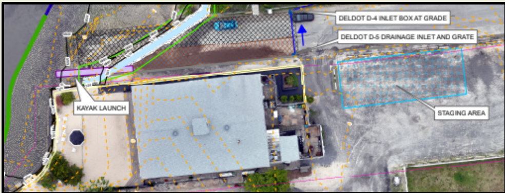
Figure 4: From the Concept Drawing, asphalt at Dagsworthy Street would be removed and replaced with a kayak launch, dune and marsh
