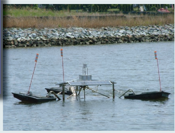
“Solar Bee” aeration system
