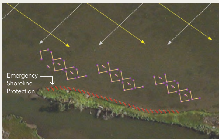
The project design uses logs to create a breakwater to reduce the wave energy hitting the shoreline.
