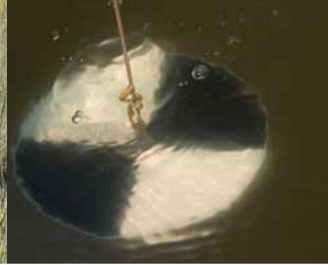
A secchi disk is used to determine the transparency—or turbidity—of water.
