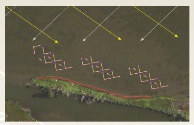
To protect this strip of eroding shoreline from prevailing winds from the northwest and storm energy from the northeast, thirty-nine 20-foot logs were fastened to the bottom offshore to create a series of three 'breakwaters.' Along the shore, with help from CIB volunteers, a series of 'cells' were built of logs and coconut fiber bio-logs to capture sediment to re-build the marsh shoreline.
